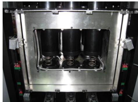
Optional Temperature controlled air heating unit (Up to 230 degrees C)
